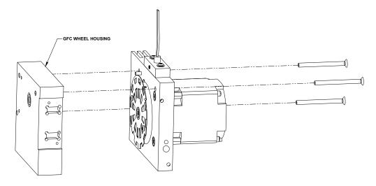
Figure 12-17: Removing the GFC Wheel Housing
